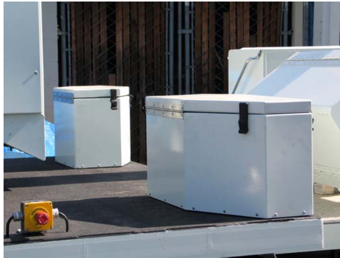
Figure 2. Radiological Threat Identification System (RTIS) on a Mobile GaRDS truck.
