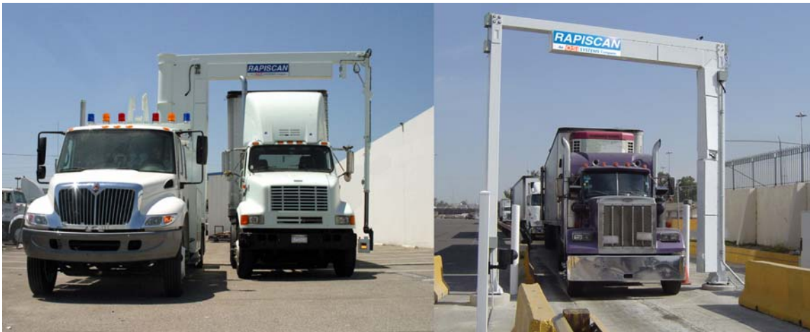
Figure 1. Mobile Gamma Radiography Detection System (GaRDS) inspecting a truck (left), and Portal GaRDS at a border crossing inspecting trucks in drive-by mode (right).
