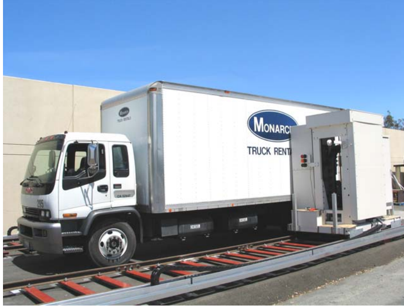
Figure 7. Portal VEDS™ scanning a truck for terrorist threats.
