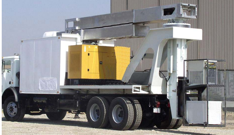
Figure 4. Highly mobile MXRVS 2-4 MeV x-ray inspection truck.
