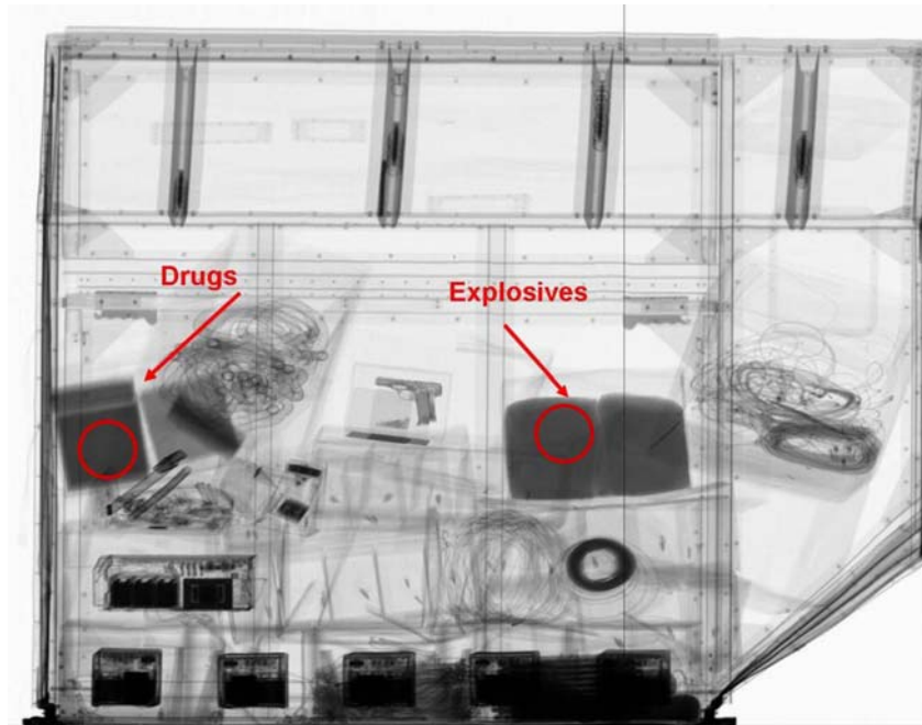
Figure 9. X-ray and VEDS™ scan of an air cargo container detect weapons, drugs and explosives.
